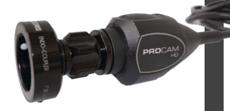
The Ecleris ProCam HD is a single chip CCD with 1280 x 720 lines of resolution and produces clear sharp images that were once only available on higher priced systems found in the surgical suite. Advanced features on the ProCam HD include Anti-moire (for flexible fiber optic endoscopes) and stroboscopy (a feature which balances the light used when performing video stroboscopy). With 3 HDMI outputs you can easily run multi video monitor configurations from a single platform.
