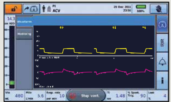
Real-time pressure and flow waveforms display essential therapy parameters on the large touch screen and allow detection of patient-device asynchrony.
